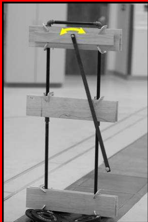
Single Pendulum: requires only one angle to specify position.
