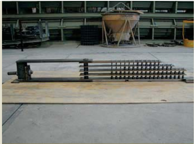
Figure 19. The prototype deviator for a curved NU I-girder consisted of four components: five straps with four layers of rollers, a solid round steel tie to hold the straps, a holding plate and end plate to transfer pull force, and a high-strength steel threaded rod to transfer the pull force to the support. Note: NU = Nebraska University.
