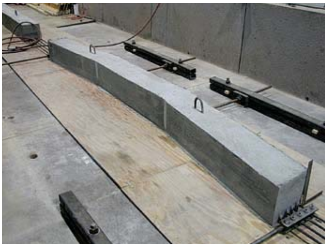
Figure 14. The test beam was cured for 26 hours before the prestressing strands were released.
