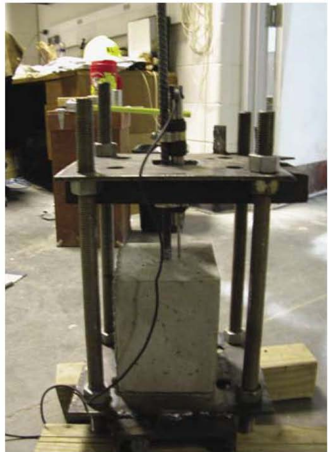
Fig. 11. Pullout test setup – Method 1.
