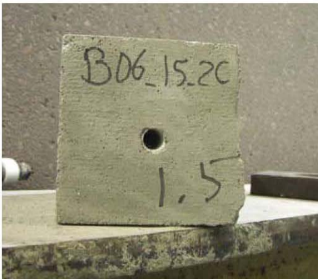
Fig. 22b. Pullout failure.
