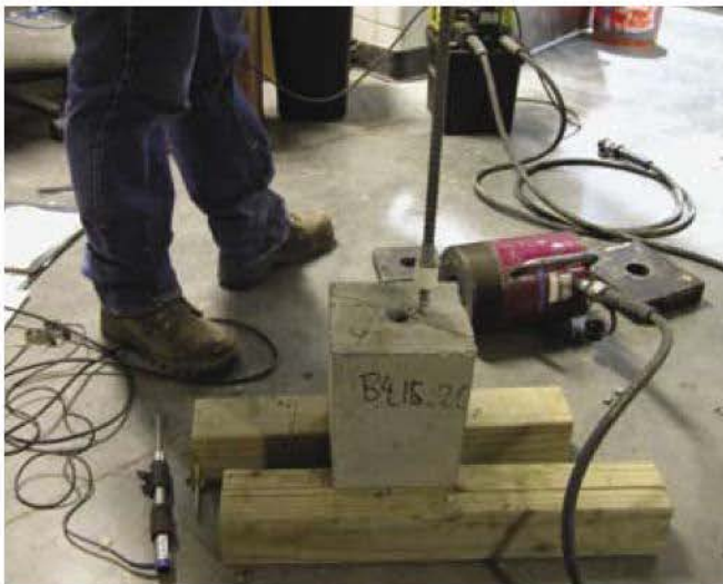
Fig. 22a. Pullout failure.
