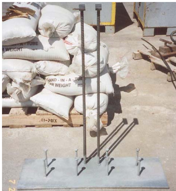
Fig. 13. Proposed end zone detail for NU-I girders.
