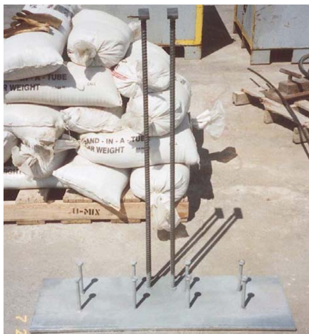
Fig. 13. Proposed end zone detail for NU-I girders.
