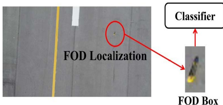
Fig. 1. The overview of the proposed FOD detection.
