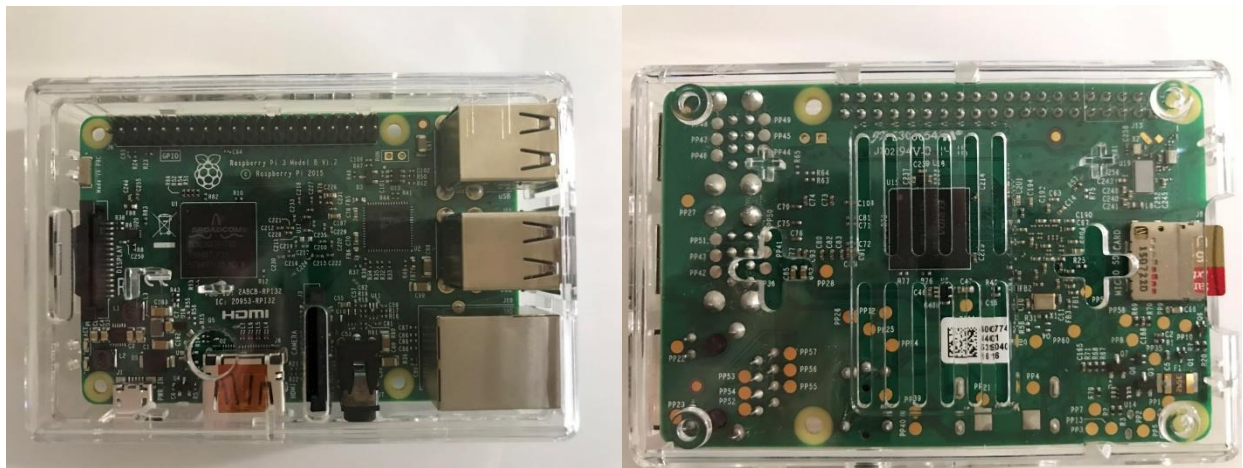
Figure 6. Raspberry Pi ® 3 Model B Motherboard
