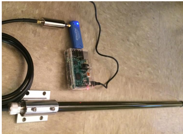
Figure 9. The Example of Assembled ADS-B Receiver
