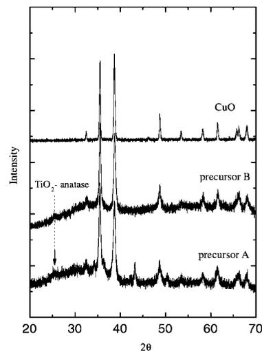
**Figure 1.** X-ray diffraction patterns of precursors A and B and commercial copper(II) oxide. Precursor A is obtained by treating the Ca/Cu/Ti/citrate gel at 450 °C for 15 min in the combustion method. Precursor B is obtained by treating a Ca/Cu/Ti/citrate/ethylene glycol solution at 450 °C for 15 min in the pyrolysis method.
