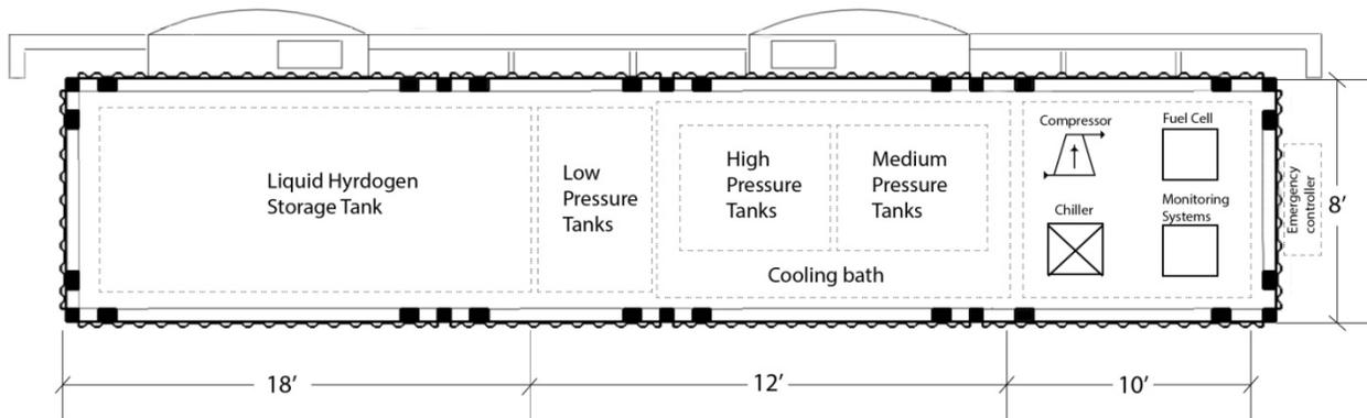
FIGURE 3. Component layout of the hydrogen station.
