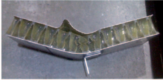
Figure 9. Failure modes observed in the flexural test.
