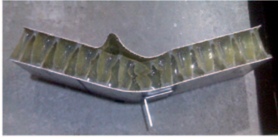
Figure 9. Failure modes observed in the flexural test.
