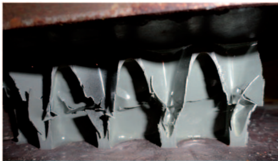
Figure 6. Failed high-impact polystyrene (HIPS) core under flatwise compression.
