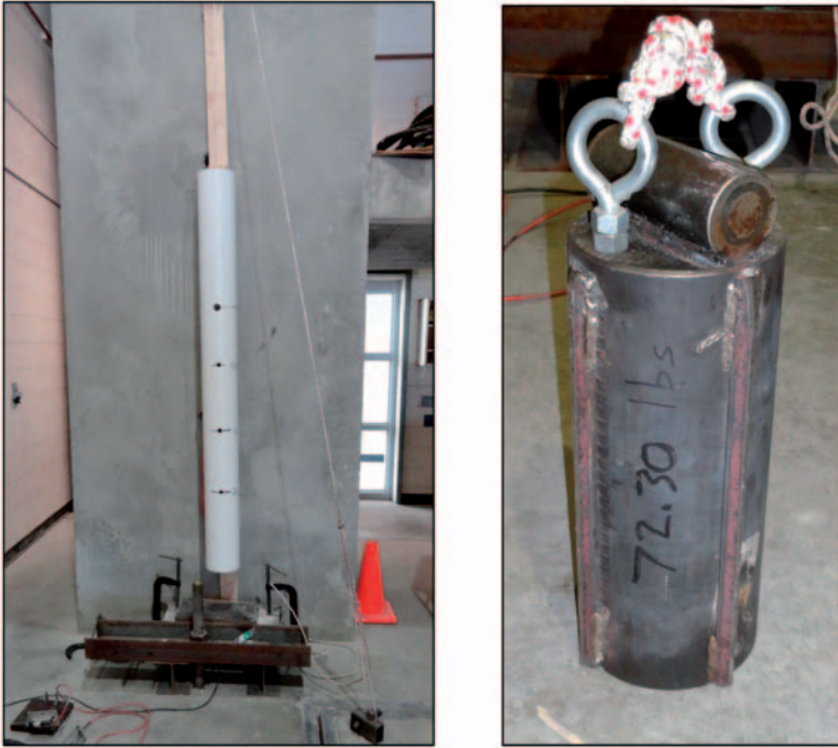
Figure 3. Drop weight testing setup.
