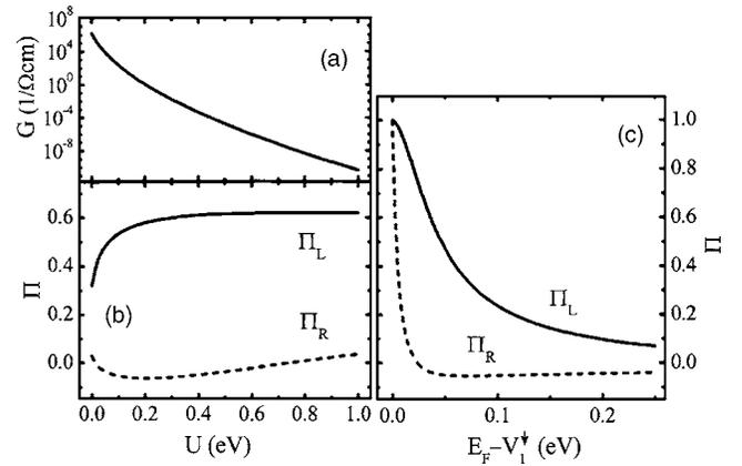
FIG. 2. Total conductance,  $G = G^\uparrow + G^\downarrow$ , (a) and spin polarization (b,c) of injected current in a DMS/FE/NS tunnel junction as a function of potential barrier height (a,b) and the Fermi energy (c) for the polarization of the ferroelectric barrier pointing to the left (solid lines) and pointing to the right (dashed lines) for  $d = 3$  nm. In (a) and (b)  $E_F - V_1^\dagger = 0.06$  eV and  $V_1 = V_2$ ; in (c)  $U = 0.5$  eV and  $V_2 - V_1^\ddagger = 0.025$  eV.
