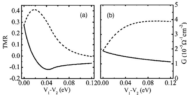
FIG. 3. Tunneling magnetoresistance (a) and conductance,  $G$ , for parallel magnetization of the electrodes (b) in a DMS/FE/DMS tunnel junction versus potential difference in the two magnetic semiconductors for the electric polarization of the ferroelectric barrier pointing to the left (solid lines) and pointing to the right (dashed lines) for  $d=3$  nm and  $U=0.5$  eV.
