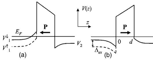
FIG. 1. Schematic representation of the potential profile,  $V(z)$ , in a DMS/FE/NS tunnel junction for the electric polarization pointing to the left (a) and to the right (b). The dashed and solid lines show the potential seen by the majority- and minority-spin carriers respectively. The horizontal solid line denotes the Fermi energy,  $E_F$ .
