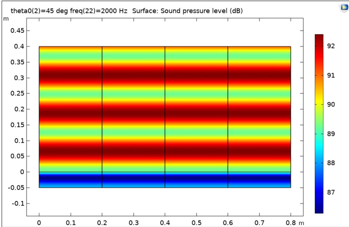
**Figure 5.** Sound pressure level plot at 2000 Hz from Porous Absorber.
