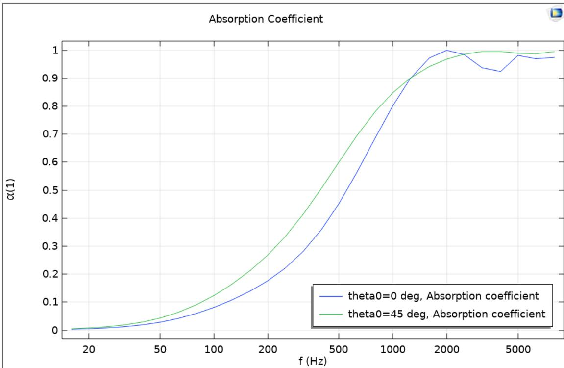
**Figure 6.** Absorption coefficient plot from Porous Absorber.
