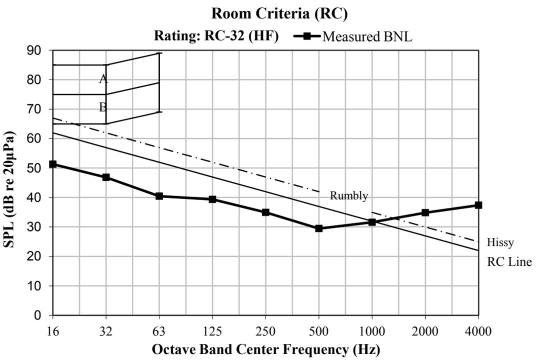
Figure 5 – RC Mark II Chart with Measured BNL
