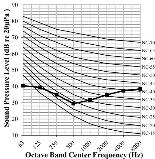
**Figure 4** – NC Rating Chart with Measured BNL
