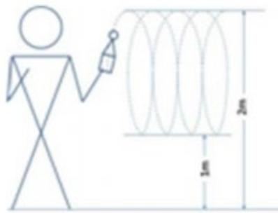
**Figure 3** – ANSI-ASA S12.71 Recommended Measurement Technique
