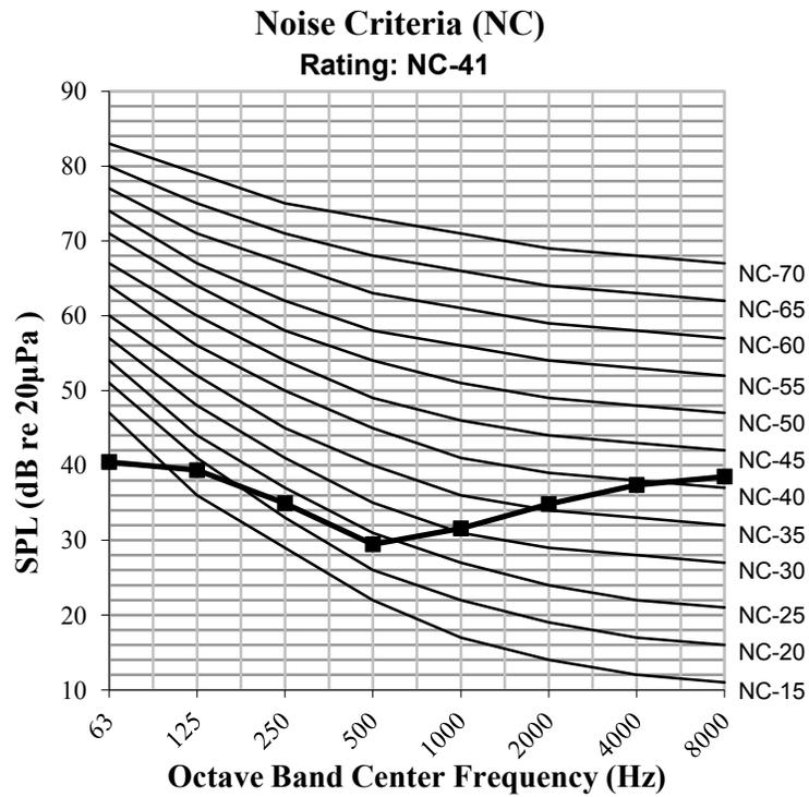
**Figure 1 - NC-Rating Chart with measured BNL**
