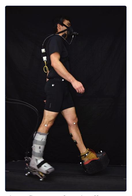
The influence of push-off timing in a robotic ankle-foot prosthesis on the energetics and mechanics of walking
