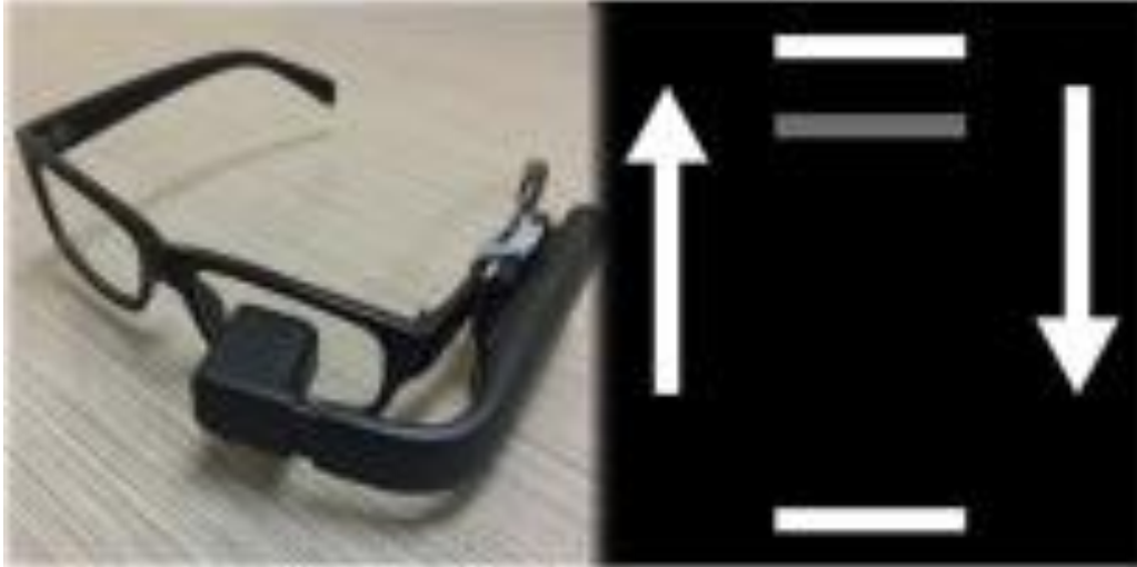
Fig. 1. Experimental apparatus (left) and the continuous visual stimulus (right) used. A miniaturized display was attached to a standard or participant's glasses, as illustrated. Note that the miniaturized display does not cover the whole lenses and was placed only on one side, allowing the subject to explore the surrounding environment while viewing the continuous stimulus. The visual stimulus (right) consisted of a grey bar moving from top to bottom and the participants were instructed to match the heel strikes of their right foot to the top and left heel-strikes with the bottom of the bar's path. The white arrows present on the figure are only illustrative of the bar's movement direction.
