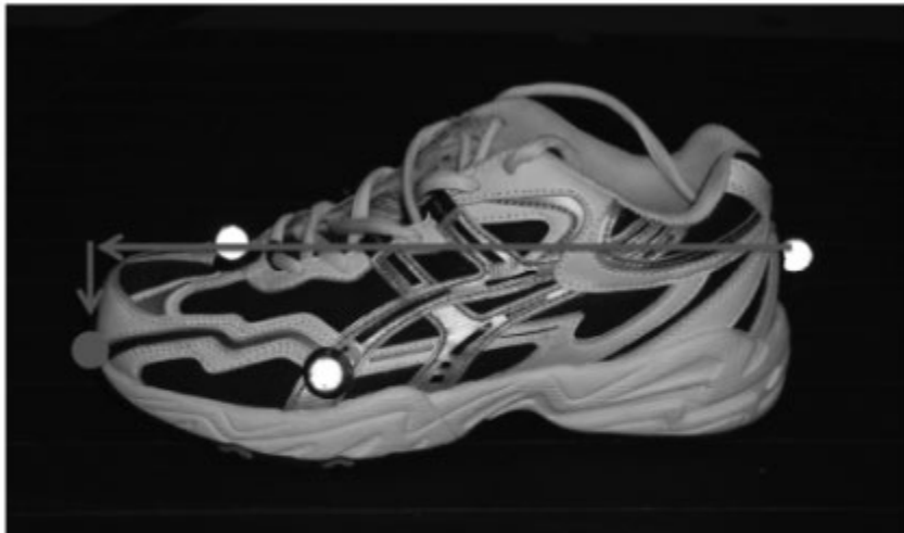
Fig. 1. Illustration of the calculation of minimum toe clearance. A virtual marker was created using Cortex (Motion Analysis Corporation, Santa Rosa, CA) software. A position was calculated by projecting a line from the heel marker through the toe marker for the length of the shoe. From this point another line was projected toward the plantar surface of the shoe the distance to the floor where the toe marker was created.
