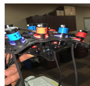
We experimented with soft plastics such as nylon to introduce advantageous flexibility throughout the cap and achieve objective two, making it more versatile. By keeping the new device flexible, theoretically it had the variability to fit the contours of each subjects skull. A disadvantage of this new design is the possibility of gap junctions between the probes and the skull. These gaps would interfere with data collection.
