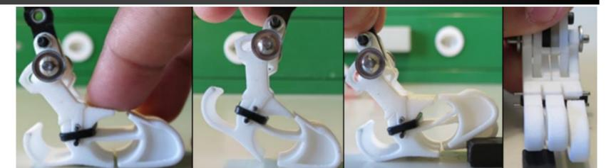
**Figure3.** Flexible foot prototype performing adaptation to different surface to manually applied force. Adopted from [3].
