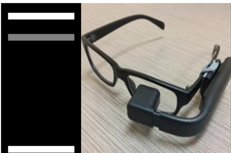
**Figure 2. a.** pacing signal viewed by participants. The grey bar moves up and down, turning red at the top to indicate when right heel strike should occur and **b.** The glasses with HDMI attachment.
