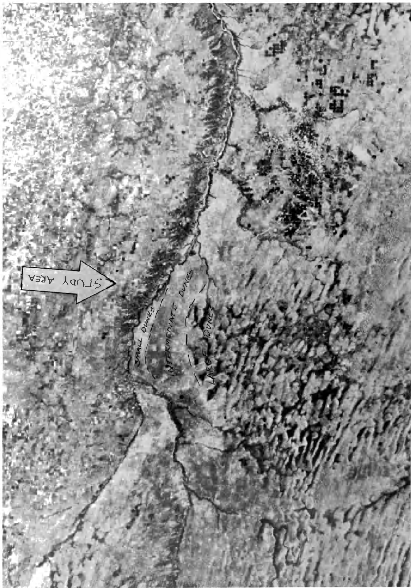
Figure 11 - ERTS image showing broad, upland, dune-mantled terraces south of the Niobrara River. The scale is approximately 1 cm = 5.6 km.
