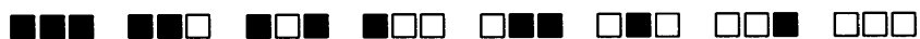
Figure 1.1: Elementary cellular automata input structure for a possible transition function. White indicates the cell is OFF; black cells are ON.
