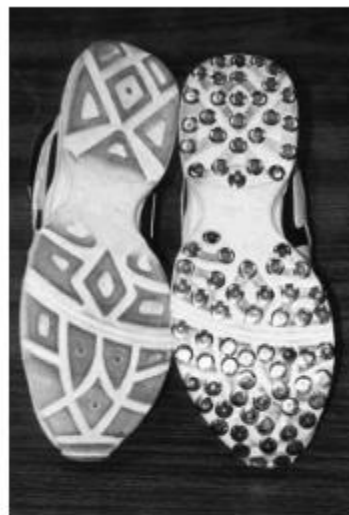
Figure 2. Soles of the high traction shoe (left) and the low traction shoe (right). The shoes (size 10) are regular running shoes (Pro-wing Joggers, 0456-2011-09-04). One pair of the shoes was altered to decrease its coefficient of friction by inserting 88 metallic one-half inch diameter disc thumbtacks into the outsole.
