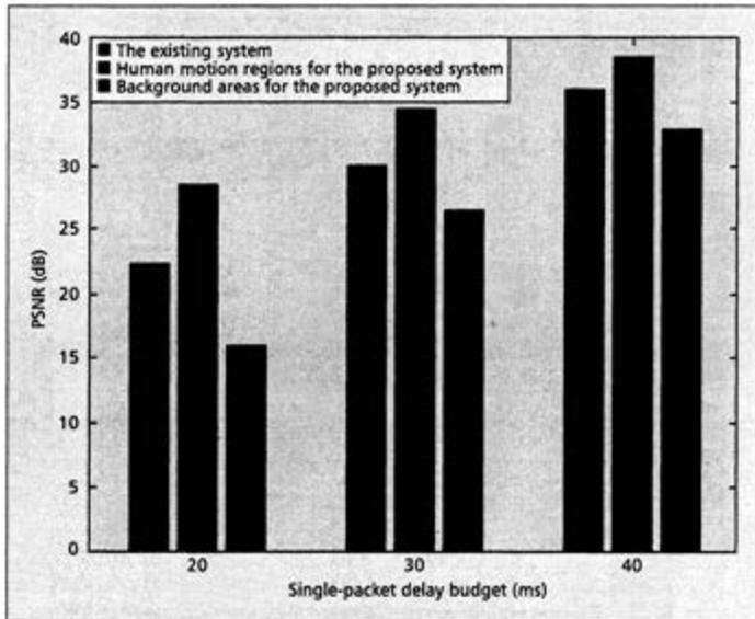
Figure 6. PSNR comparison of different single-packet delay deadlines.
